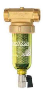
Mini Cleaning Filters - Sand collector self cleaning filter with brass head and ring nut. Stainless steel cartridge. It cleans as it is equipped with a drain valve that removes the sand without having to take apart the filter.
