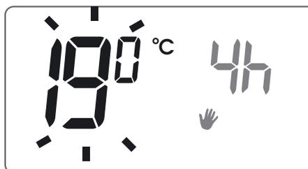
If the selection is not confirmed within 10 seconds, the regulator will automatically enter vacation mode.
