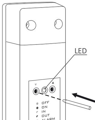
1. The process of pairing the **2025 RTH** regulator with the **RTH** receiver is initiated by pressing the left pairing button (marked with a green triangle - ▼ ) on the **RTH** receiver and holding it for at least 2 seconds, until the LED starts flashing green, and then releasing the button.
