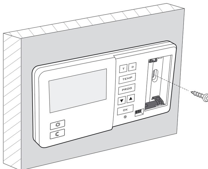
**NOTE:** If the wall is wooden, there is no need to use wall plugs. In such a case, drill two holes 2.7 mm in diameter instead of 6 mm, and screw the screws directly into the wood.
