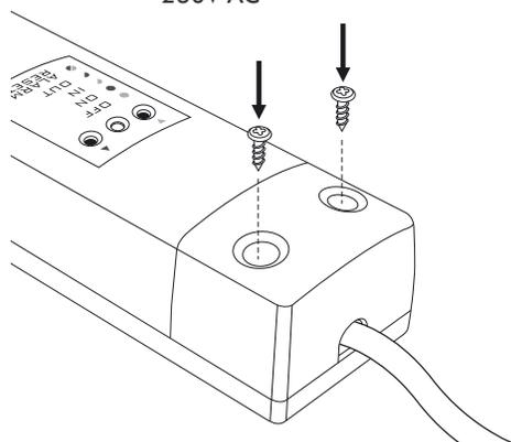
5. After connecting the conductors, they must be secured with the cable tie clamps and reinstall protective covers of the **AURATON RTH** receiver.
