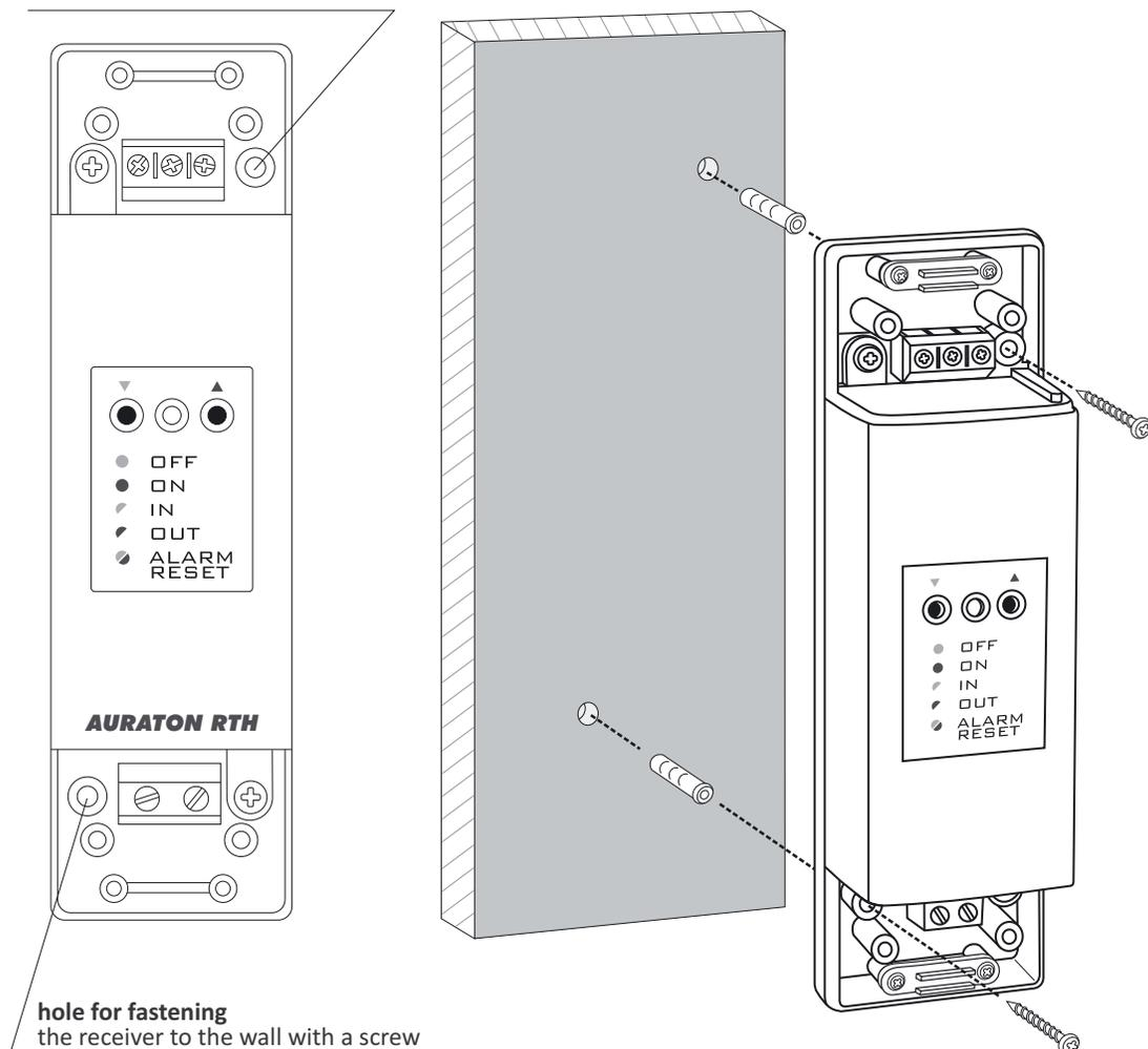
**NOTE:** If the wall is wooden, there is no need to use wall plugs. In such a case, drill two holes 2.7 mm in diameter instead of 5 mm, and screw the screws directly into the wood.
