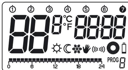
Following that, the regulator enters time setting mode; the hour field flashes, prompting for setting it.
