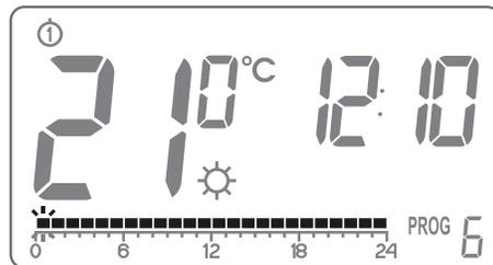
4. All (24) rectangles will be lit on the time line. One rectangle corresponds to one hour. If a rectangle is visible, the day temperature will be maintained during the corresponding hour. A turned off rectangle indicates that the night temperature will be maintained. In the picture, the first rectangle flashes - a flashing rectangle indicates the point on the time line where the change is being made.
