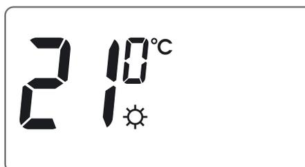
3. Using the **▼** and **▲** buttons, set the desired temperature setpoint.
