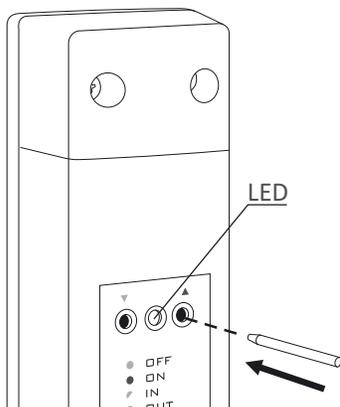
1. Deregistering the **2025 RTH** regulator from the **RTH** receiver is initiated by pressing the right deregistering button (marked with a red triangle - ▲ ) on the **RTH** receiver and holding it for at least 2 seconds, until the LED starts flashing red, and then releasing the button.
