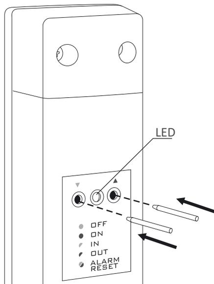
In order to deregister all devices paired with the RTH receiver, simultaneously press both the pairing and the deregistering button ( ▼ and ▲ ) and hold them for at least 5 seconds until the LED flashes alternating red and green. Then release both buttons.
