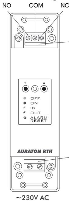
3. Connect the heating device to the **control connection terminals** of the **AURATON RTH** receiver. Proceed in accordance with the service manual of the heating device. Most commonly, the **COM** (common) and **NO** (normally open) terminals.
