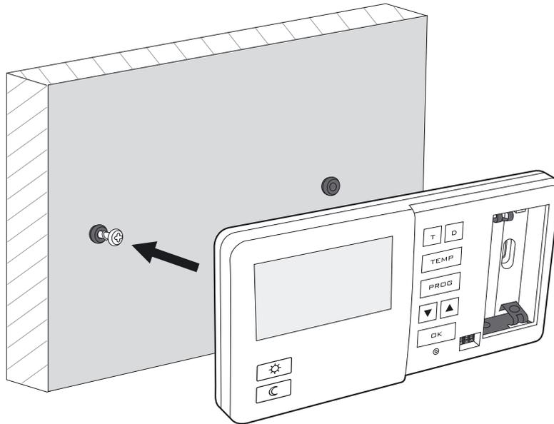
5. Screw in the right screw, making sure it holds the regulator securely.
